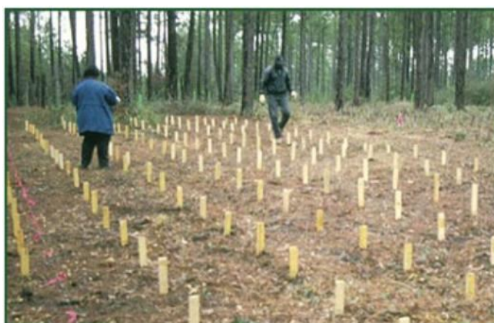
Figure 9. Inground stake test.
