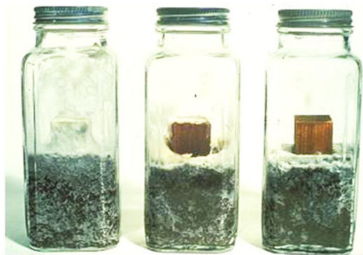
Figure 4. ASTM standard soil block test.
